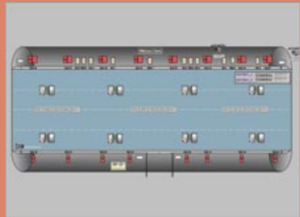
A Ventilation Control Screen for the Attiki Odos Motorway in Greece
