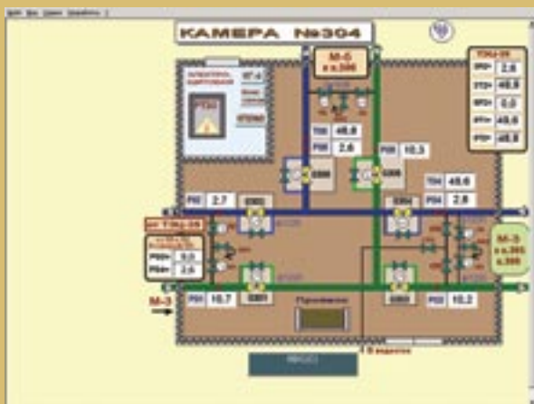
Overview Screen at Mosenergo Heating and Pipeline
