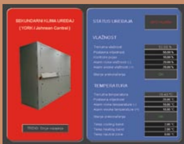
An Air Conditioner Monitoring Screen in an Example Alarm Condition
