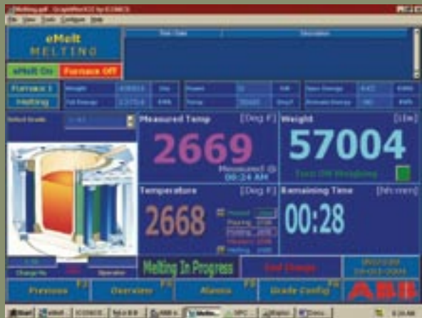
Melting Control Screen at ABB Foundry Group
