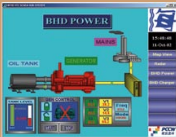
Generator System Display at the Hong Kong Marine Department
