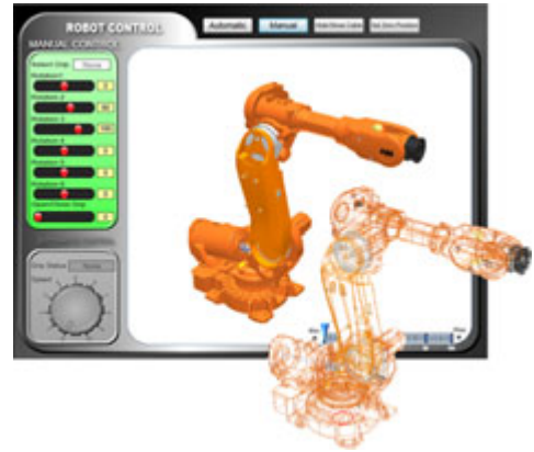
Fig. 14. 3D drawings imported in ICONICS HMI
